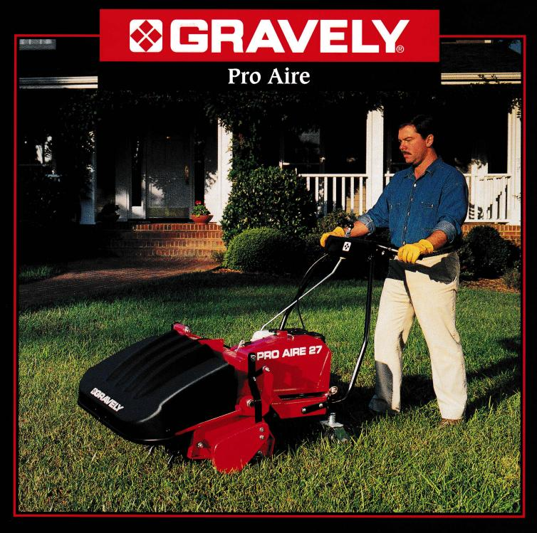
The Gravely Pro Aire 27 is as easy to operate as a mid-size rotary mower. The hydraulics allow the operator to switch from aeration to transport with the touch of a lever. This feature makes operation easy by not requiring lifting and pushing around trees, bushes, and other obstacles. The Pro Aire 27 is equipped with an Automatic Weight Transfer system that keeps the weight and balance where needed for transport or aeration.
